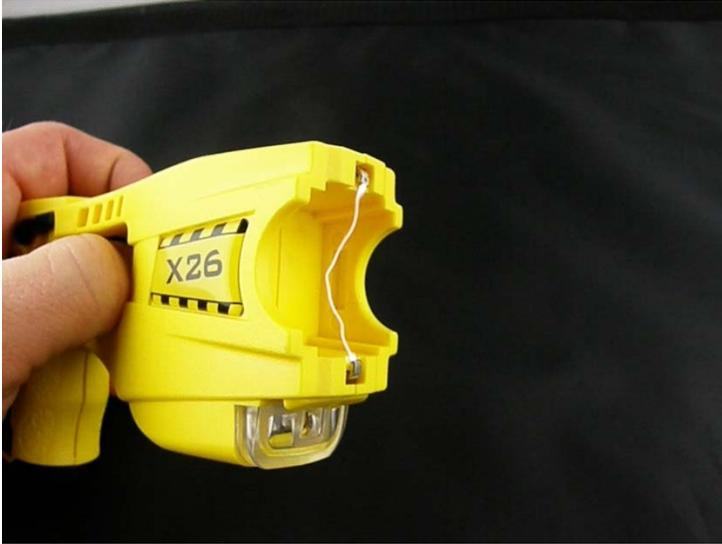
Electricity arcing between fixed electrodes on CEW without a cartridge attached
