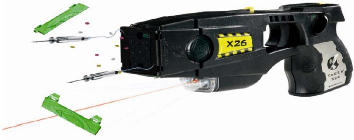
CEW probes deploying through green blast doors
